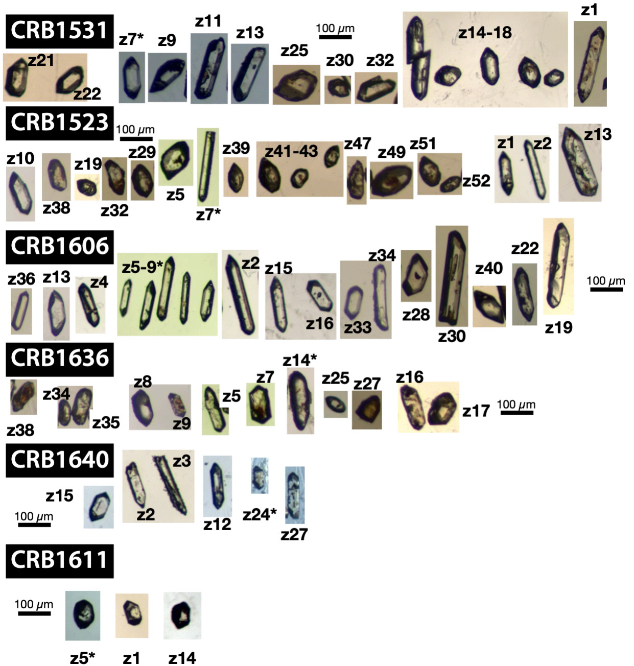
Fig. DR2. Zircon Photos. Optical images of zircons under transmitted light are presented here, with stratigraphic younging from bottom to top. Zircons present a range of morphologies, but the majority are euhedral with sharp crystal terminations, indicating an igneous rather than detrital origin. The zircon yielding the youngest, most precise analysis for each sample is starred.
